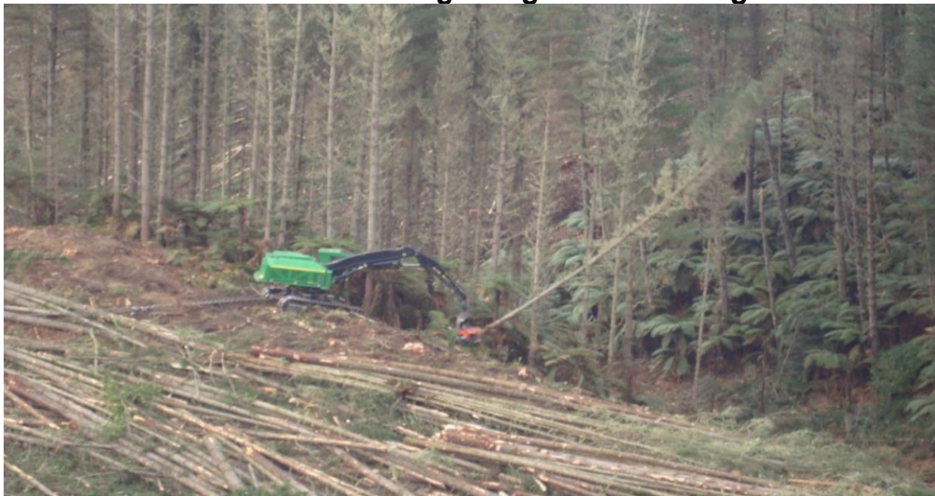
Photo: Tethered mechanised harvesting using a self-levelling machine
