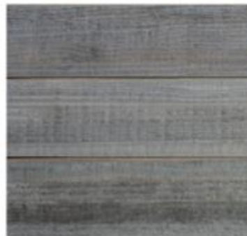
Graphite weathered after 6 months
