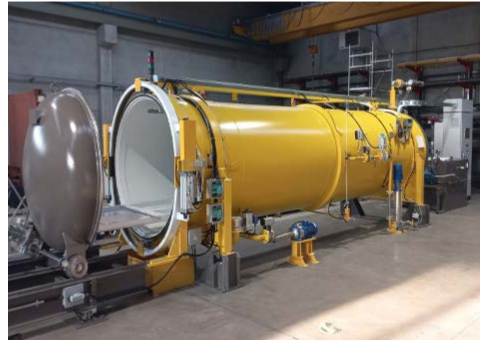
○ Vaaro treatment pressure vessel.
