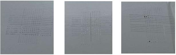
Very little to no delamination along edges or at intersections. ISO class 0/1. Very small area where water had been allowed to penetrate and absorb into the timber can any surface timber weakness be seen (common with thermally modified timber).
