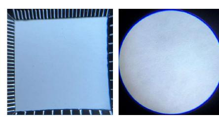
When viewed under magnification, the coating appears sound with good flow into any open pores of the timber.
