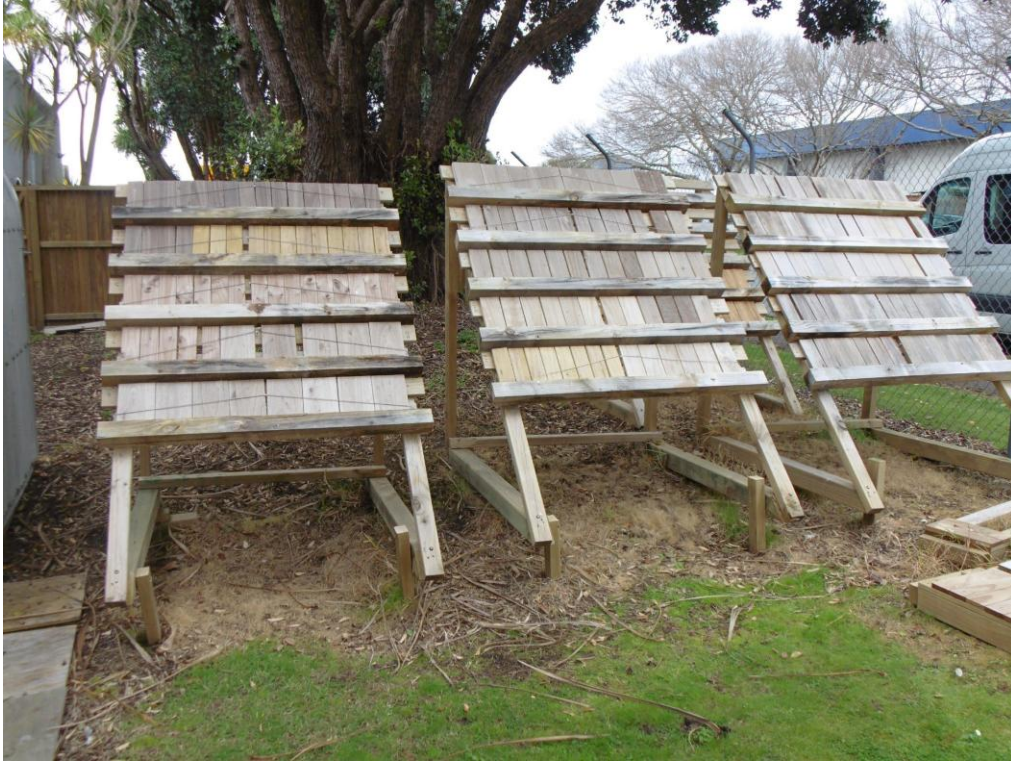
A-frame test racks for exposure of samples T at first inspection time
