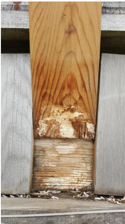
Western red cedar decay on back of sample and supporting panel/rack (17 months exposure)
