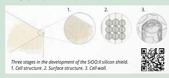
The SiOO:X system mechanically prevents microorganisms from establishing themselves inside the wood. The protective silicon shield inside the wood fibers takes different lengths of time to develop. 0–12 months for decking and 0–4 years for cladding. The fact that SiOO:X develops over time also means that its resistance to staining by black spores and the like improves with time, unlike traditional surface treatment products.
