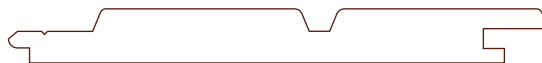
WB10FP 180x18 (160mm cover) Supplied as a custom profile. Order subject to minimum order quantity and lead time.
