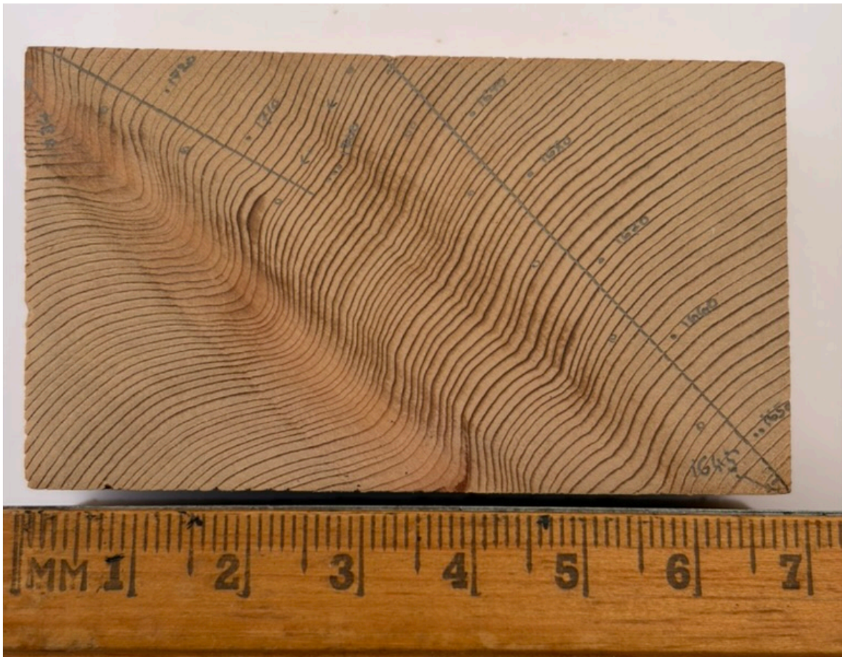
Figure C3: Image of ABD03. The growth direction is from the bottom to the top of the image. Note, ring deformation usually caused by nearby branching.
